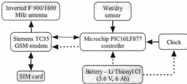
Figure 1. Schematic diagram of phone-tag. The dotted lines show power. The solid lines show data flow.
